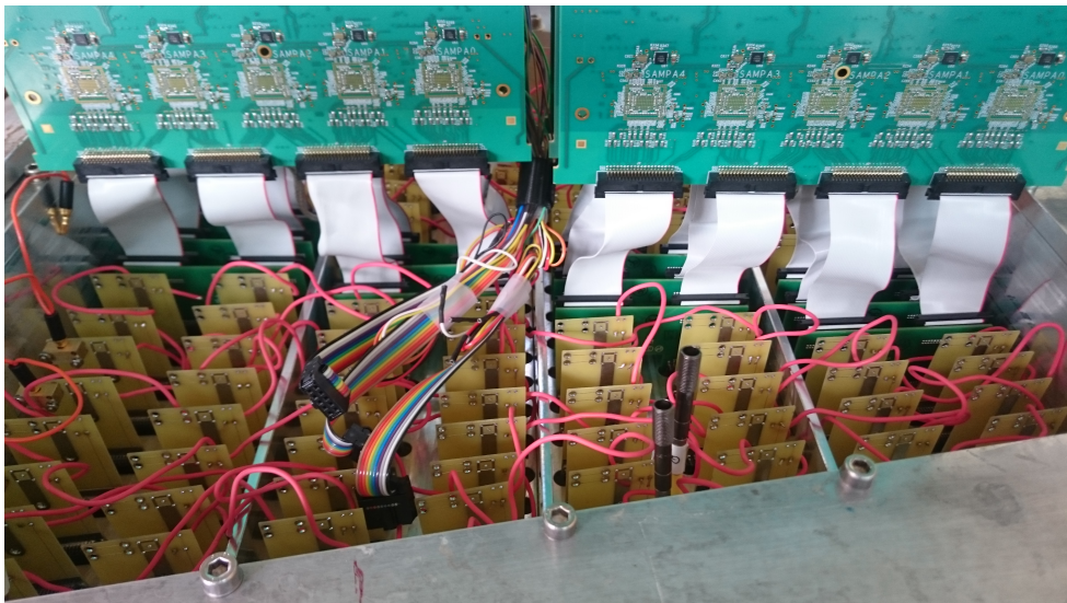
Figure 4.2: Close view of the connections to the readout anode. The front-end cards (green) with SAMPA chips are connected to a sub-set of the pad plane of the IROC. Grounding cards (yellow) define the potential of the remaining part of the pad plane.
