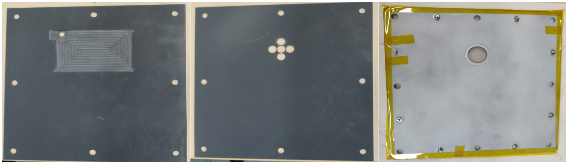
Figure 2.12: Different sample holder types: sample holder for metal plates (left), sample holder for the frames (middle), sample holder for glass window (right)
