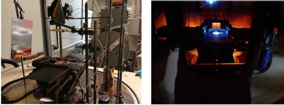
Figure 2.9: Interior of the coating chamber with an inserted THGEM (left), and a picture taken during the coating procedure where the blue glowing circle is the CsI pill(right). The right side picture is taken from [47]
