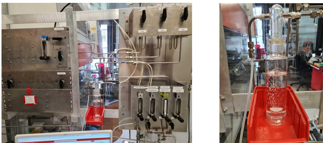
Figure 2.1: A picture of (a) the gas system and (b) a close-up of the bubbler used for humidifying the gas.
