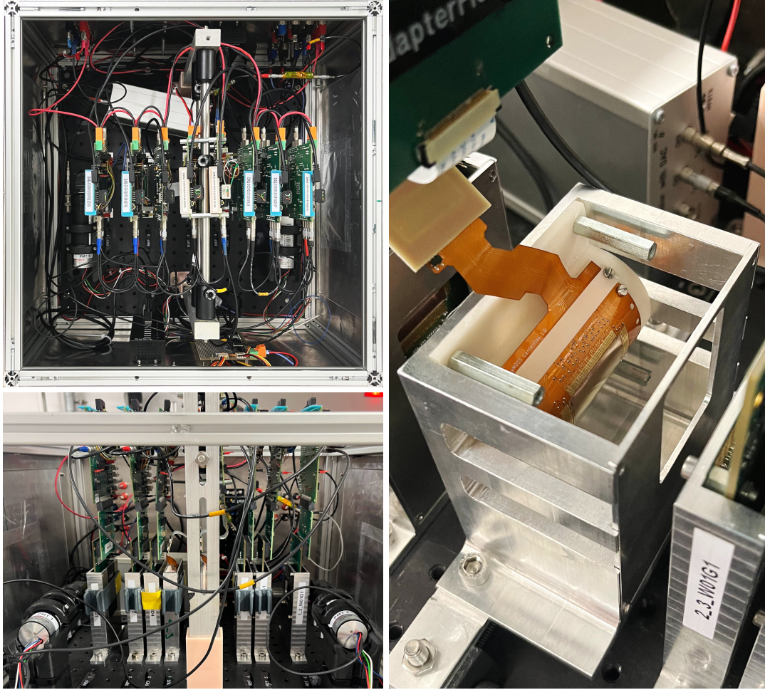
Figure 2.5: Photographs of the telescope used in the testbeam. The beam direction is from right to left. The telescope box is shown from the top (top-left) and from the side (bottom-left), where the latter view includes a second DUT that replaced the first after the Flat 1 measurement. On the right, a close-up of the DUT in the R_{\text{rows}} = 18 mm configuration is shown mounted inside the telescope.
