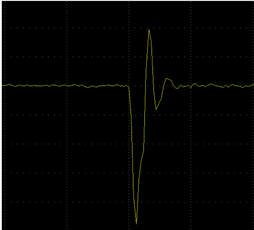
Figure 3.7: Closeup of a discharge signal induced by foil bending in the induction gap at an induction field of 11 kV/cm. The x axis displays the time divided into 100 ns divisions respectively the y axis displays the amplitude in 1.5 V divisions.
