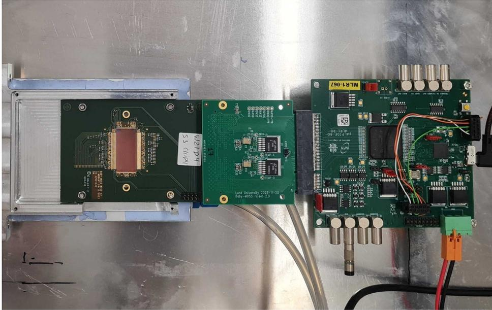
Figure 3.4: A picture of the BabyMOSS setup used for testing the sensor and performing source measurements.
