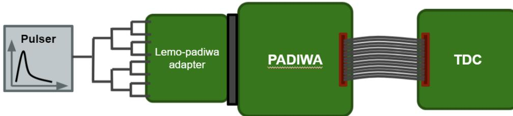
Figure 3.17: Sketch depicting the setup for measuring the relative time delays between channels for time calibration.
