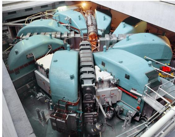
Figure 3.23: The large PSI Ring Cyclotron. The turquoise structures are the eight sector-magnets and between them in dark grey the four acceleration cavities. *Photo: Markus Fischer/ PSI*
