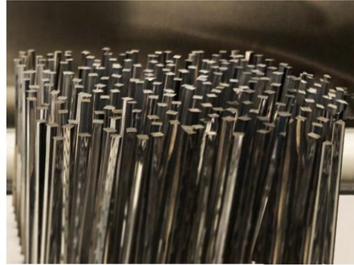
Figure 3.3: Photograph of a fiber bunch before being installed into the modules.
