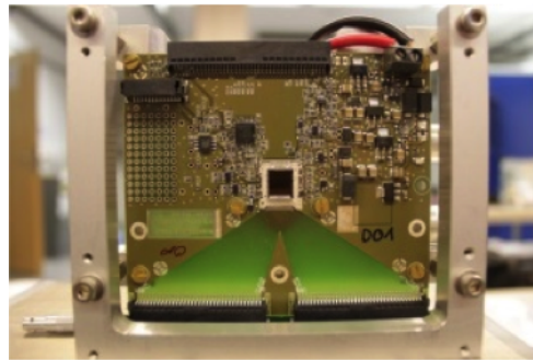
Figure 4.5: The n-XYTER ASIC chip used as front-end electronics mounted on a aluminium cooling block.
