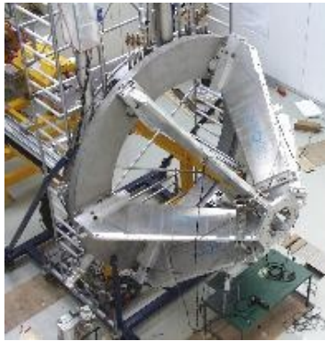
Figure 2.6: Photograph of the superconducting toroidal magnet of HADES.
