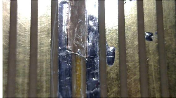
**Figure II.3:** The soldered connection of the two strip foils for the outer field cage.
